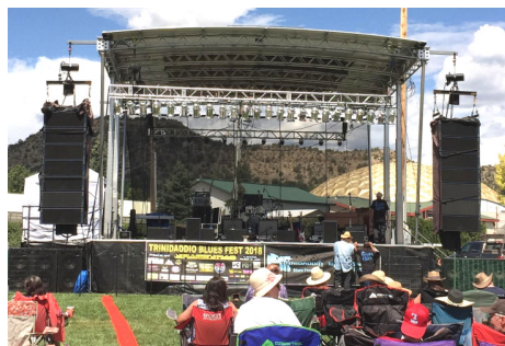
SC 48 Avid Console with 16 Box JBL Line Array Stacked System with Lighting
